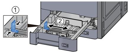
Adjust the position of the paper width guides located on the left and right sides of the cassette.
