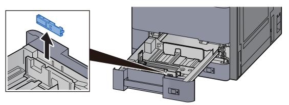
3 Expand the lever of the envelope feed guide when loading envelopes larger than Envelope C5 which has a width of 162 mm (6.4").
