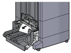
5 Open the folding unit conveyor guide.
