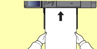
• After printing starts, catch the paper when it is output so that it does not fall. When using the inner tray as the output location, do not stand up the stopper.
