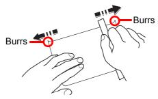
Before loading Hagaki (Cardstock), fan them and align the edges. Hagaki (Cardstock) should be fed from the MP tray with the print-side down or the cassette and the optional paper feeder with the print-side up. If the Hagaki (Cardstock) paper is curled, straighten it before loading. Printing onto curled Hagaki (Cardstock) may cause jams.
