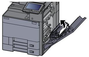
$\frac{15}{5}$  Remove the paper from the paper ejector.
