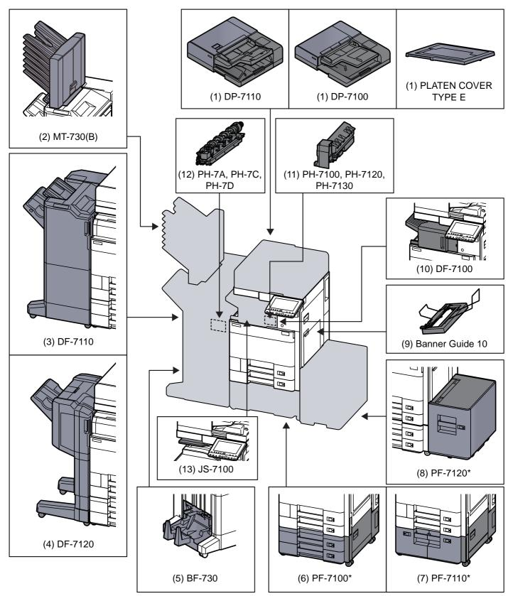
\* If the following option is installed, toppling prevention kit must be installed: PF-7100, PF-7110, PF-7120
