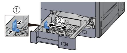
6 Adjust the position of the paper width guides located on the left and right sides of the cassette.
