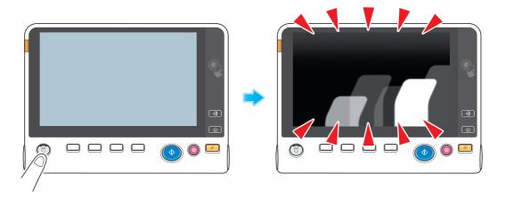
Check to see that the Main Power Switch and the Power key are turned ON.
