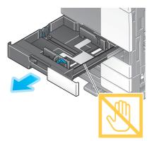
2 Slide the **Lateral Guide** to fit the size of the paper to be loaded.
