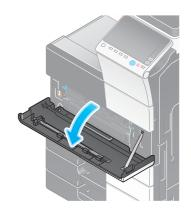
2 Release the Waste Toner Box Lock Lever, then remove the Waste Toner Box.
